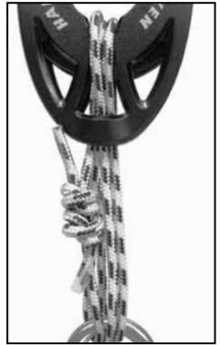
Knot can also be located on side of block or inside the mouth.
