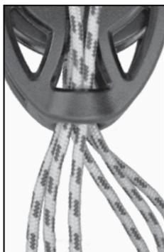
Three (3) laps, six (6) strands are required for proper strength.
